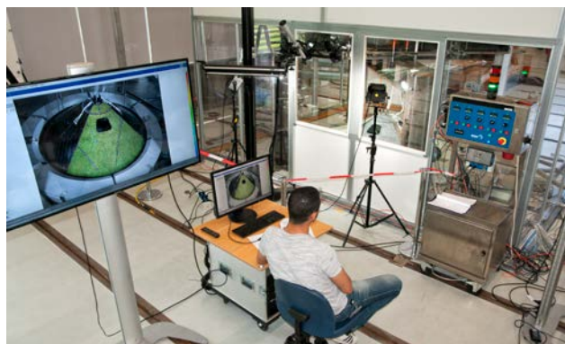
Actual full-scale space structures testing at -180^{\circ}\text{C} .
