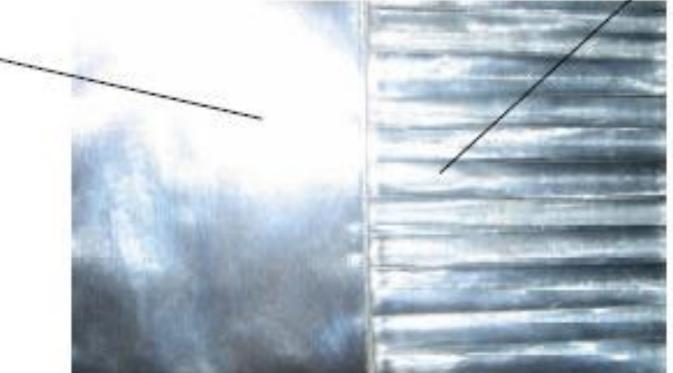
Fig.5c – Intuitive experiment done with concentrated light reflected by a flat and a corrugated surface
