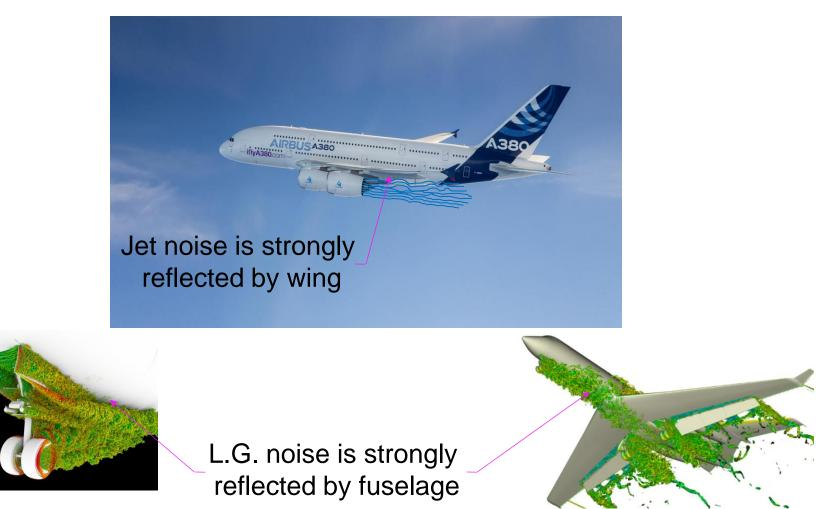
In the case of present aircraft noise generated by jet and landing gear is strongly reflected by wing and fuselage to community
