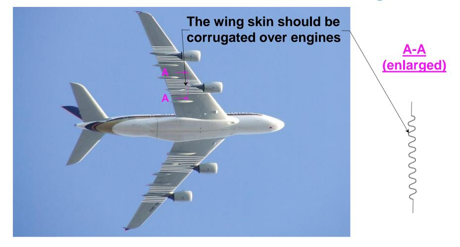
Fig. 2-Aircraft with corrugated wing skin on pressure side, over engines
