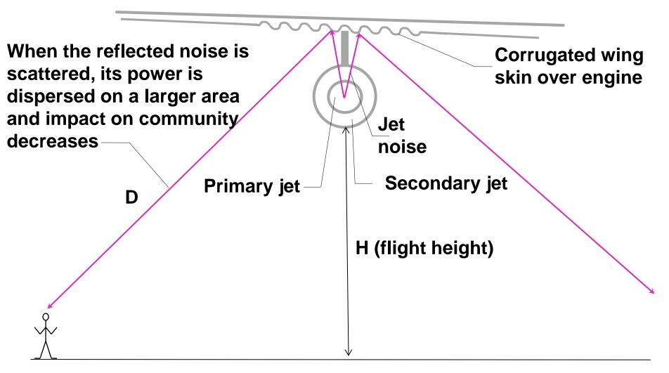
Fig.4 – The case of corrugated wing skin over engine
