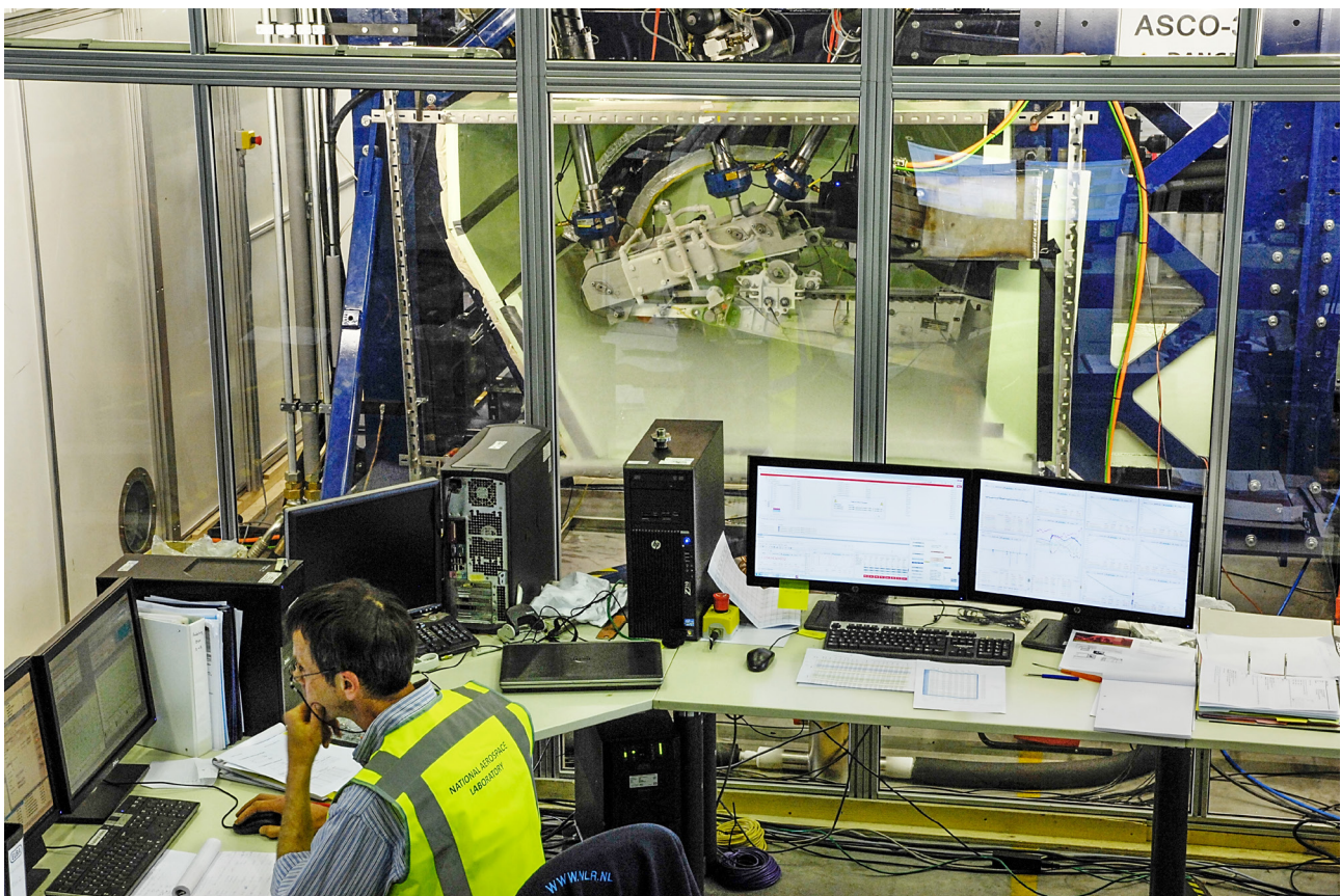
Overview of full scale flap track test setup at -55^{\circ}\text{C} .
