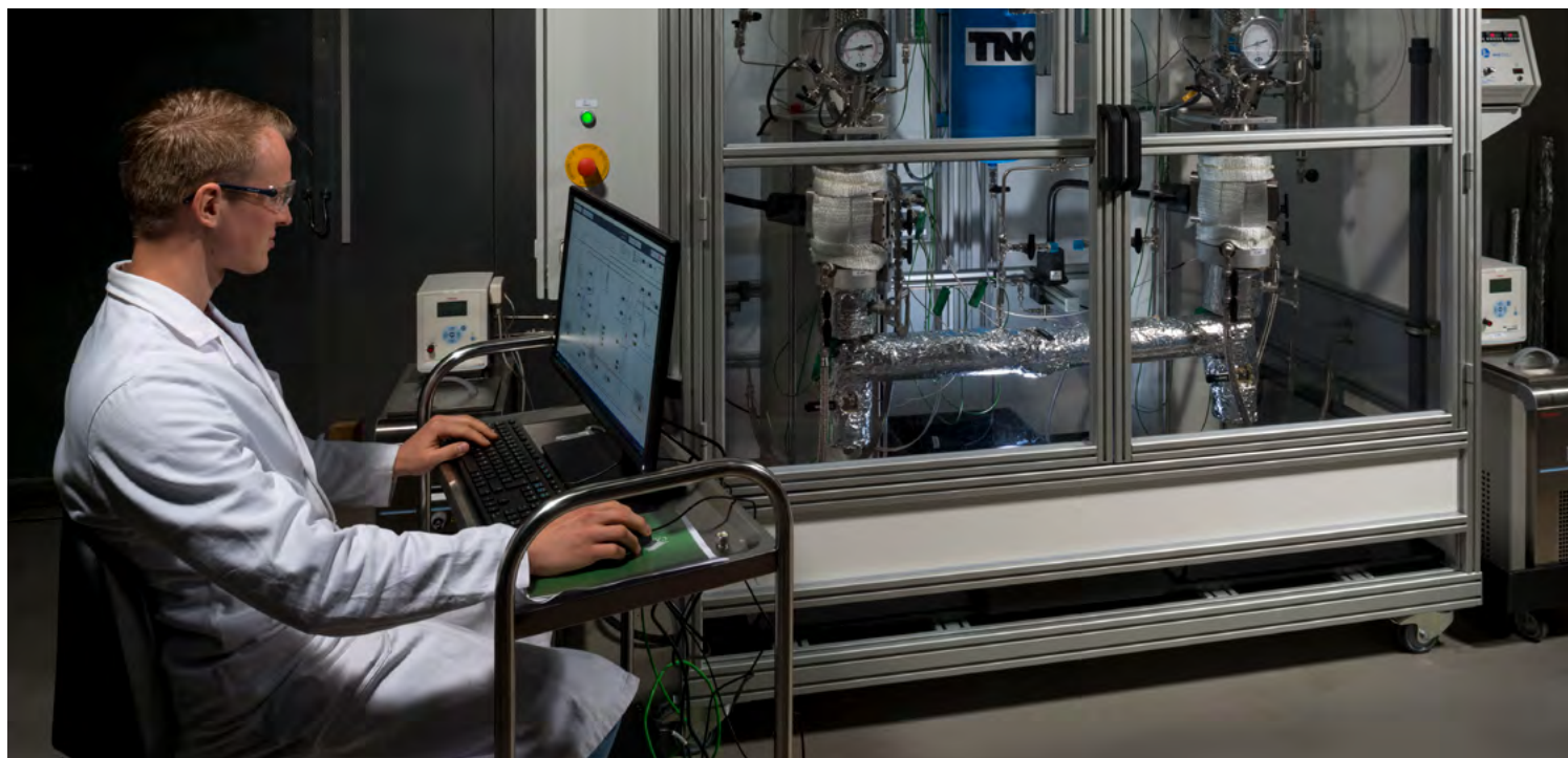
Test set-up for solvent recycling of waste plastics (dissolution).
