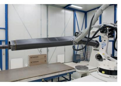
The challenge: to find out whether thermoplastic materials can be used for really thick and large components, for example in aircraft. Parts of the aircraft engine pylon become very hot during normal use of the aircraft. For that reason, the pylons currently used are commonly made of titanium. Most of the parts, such as ribs and spars in the pylon, are made by forging and milling. A reduction of costs might be achievable if the titanium parts can be replaced by composite materials.
