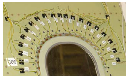
Strain gauges on window panel
