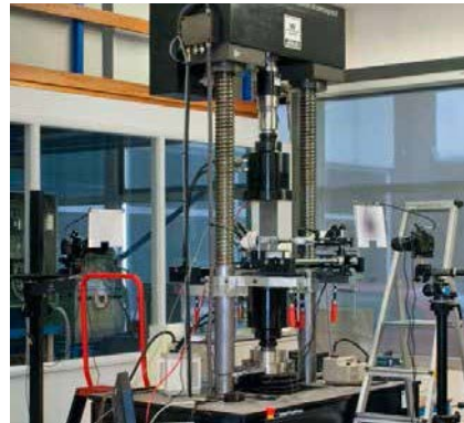
Amsler, crack growth sample, see below
