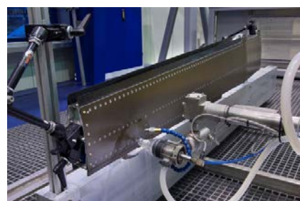
Squirter inspection large aircraft component
