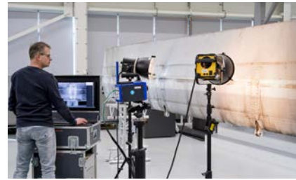
Thermography on wing flap
