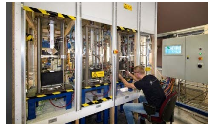
Electric and hydraulic dynamic test machines with enhanced chemical environments
