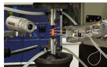
Creep test with coil heating, strain measuring and grip cooling
