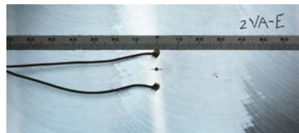
Fully automated crack growth monitoring
