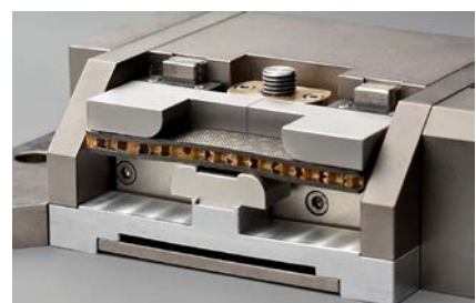
Micro mechanical test setup (four point bending)
